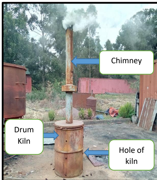
a) Carbonization of mango peel
