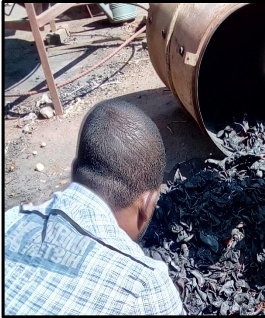
Figure3. 8: After carbonization process of mango peel product
