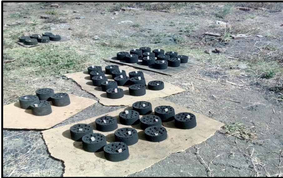
Figure3. 12: Briquette produced on sun drying
