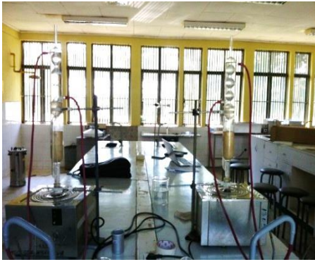
(a) Solvent method oil extraction
