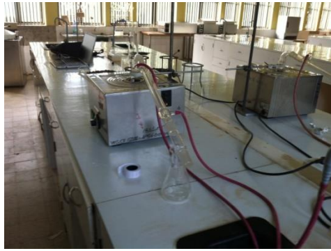
(b) Fractional distillation to recovery n-hexane
