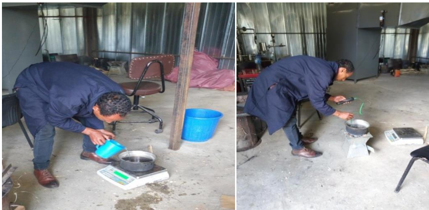
Fig 4a. Water boiling test with briquettes
