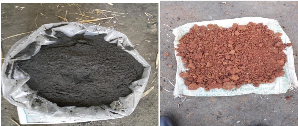
Fig 3a. Carbonized powder and clay soil binder preparation
